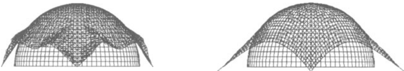
Figure 6. Simulation shape obtained with woven fabric \pm 45^\circ (a) and 0^\circ (b)
