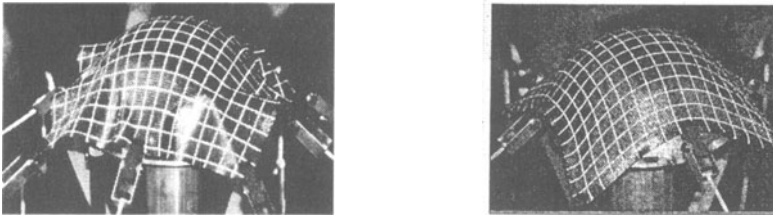
Figure 5. Experimental shape obtained with woven fabric \pm 45^\circ (a) and 0^\circ (b)
